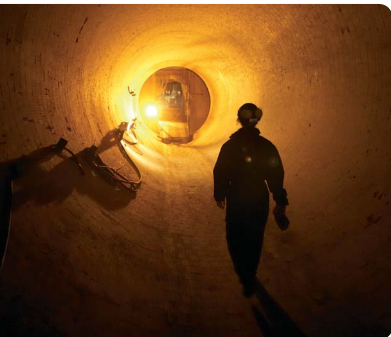
View inside a rotary cement kiln during scheduled shutdown
